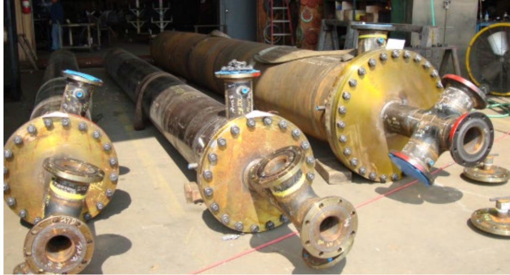
Figure 3: Conventional Sulfur seals not installed in the pit.
