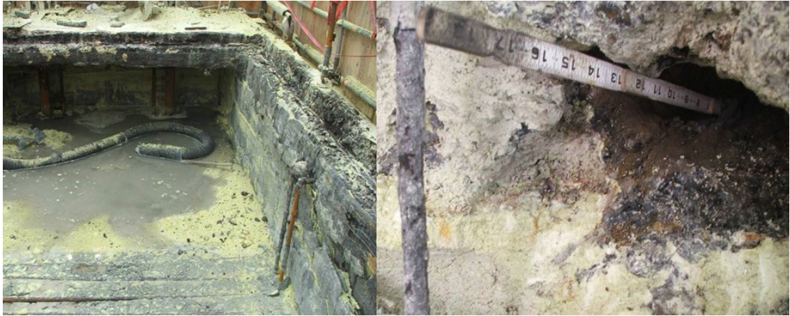
Figure 5: Sulfur pit sidewall leaking steam coil penetrations resulting in concrete degradation and reduced molten Sulfur heating efficiency.
